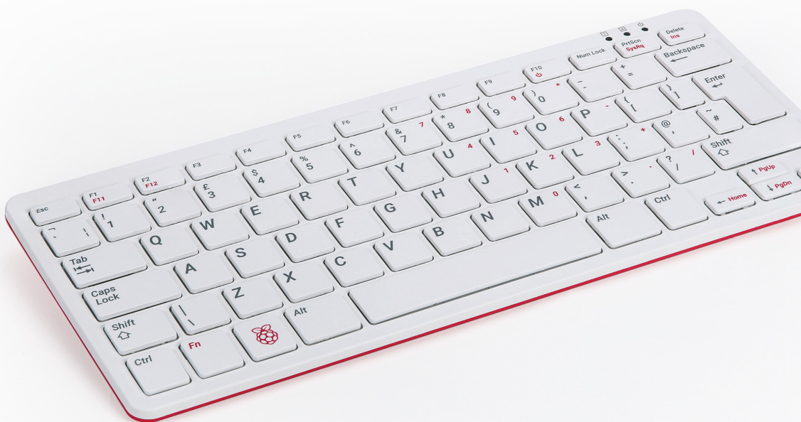
▲ Figure 1-16: Raspberry Pi 400 has an integrated keyboard
