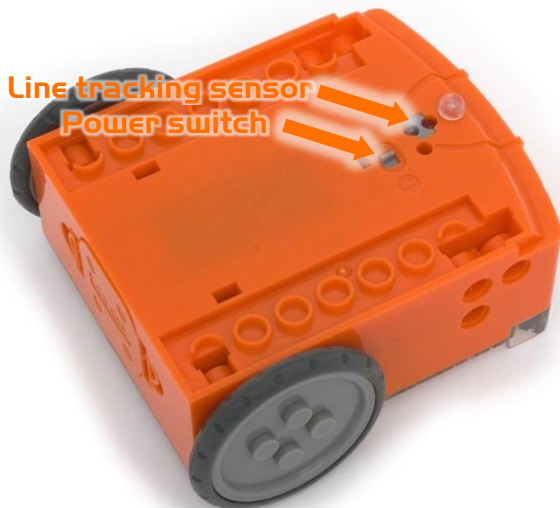
Edison's power switch and line tracking sensor
