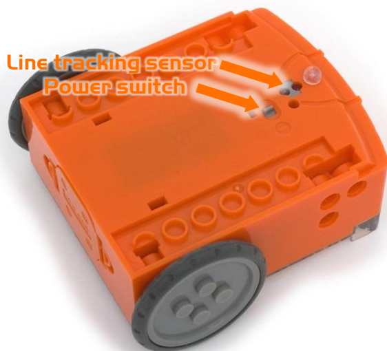
Edison's power switch and line tracking sensor
