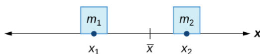
Figure 2.63 The center of mass \bar{x} is the balance point of the system.
