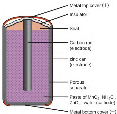
Figure 17.10 The diagram shows a cross section of a flashlight battery, a zinc-carbon dry cell.
