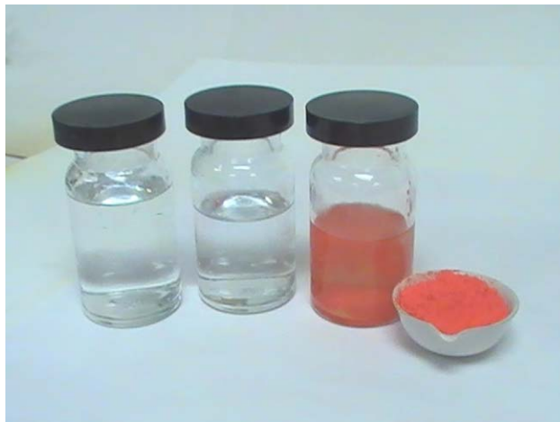
Figure 18.61 Solid HgI 2 forms when solutions of KI and Hg(NO 3 ) 2 are mixed. (credit: Sahar Atwa)
