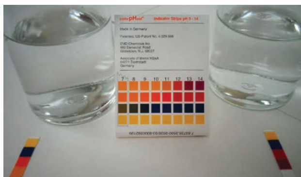
Figure 14.10 pH paper indicates that a 0.1- M solution of \text{NH}_3 (left) is weakly basic. The solution has a pOH of 3 ( [\text{OH}^-] = 0.001\text{ M} ) because the weak base \text{NH}_3 only partially reacts with water. A 0.1- M solution of \text{NaOH} (right) has a pOH of 1 because \text{NaOH} is a strong base. (credit: modification of work by Sahar Atwa)
