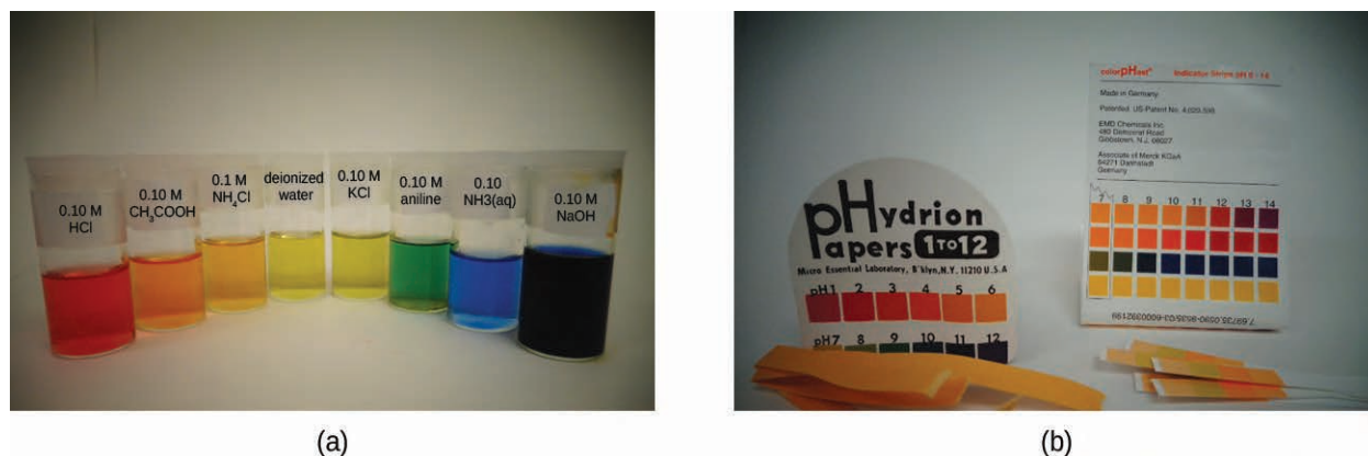
Figure 14.5 (a) A universal indicator assumes a different color in solutions of different pH values. Thus, it can be added to a solution to determine the pH of the solution. The eight vials each contain a universal indicator and 0.1-M solutions of progressively weaker acids: HCl (pH = 1), \text{CH}_3\text{CO}_2\text{H} (pH = 3), and \text{NH}_4\text{Cl} (pH = 5), deionized water, a neutral substance (pH = 7); and 0.1-M solutions of the progressively stronger bases: KCl (pH = 7), aniline, \text{C}_6\text{H}_5\text{NH}_2 (pH = 9), \text{NH}_3 (pH = 11), and NaOH (pH = 13). (b) pH paper contains a mixture of indicators that give different colors in solutions of differing pH values. (credit: modification of work by Sahar Atwa)
