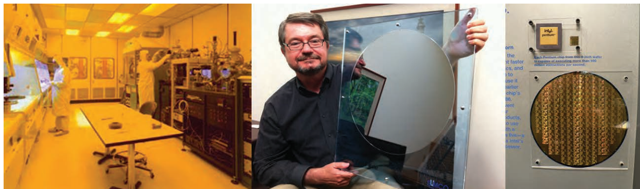
Figure 18.1 Purity is extremely important when preparing silicon wafers. Technicians in a cleanroom prepare silicon without impurities (left). The CEO of VLSI Research, Don Hutcheson, shows off a pure silicon wafer (center). A silicon wafer covered in Pentium chips is an enlarged version of the silicon wafers found in many electronics used today (right). (credit middle: modification of work by “Intel Free Press”/Flickr; credit right: modification of work by Naotake Murayama)
