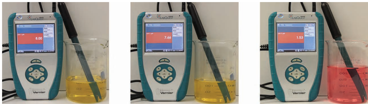
Figure 14.19 The indicator color (methyl orange) shows that a small amount of acid added to a buffered solution of pH 8 (beaker on the left) has little effect on the buffered system (middle beaker). However, a large amount of acid exhausts the buffering capacity of the solution and the pH changes dramatically (beaker on the right). (credit: modification of work by Mark Ott)
