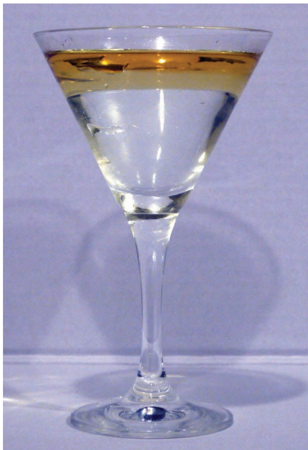
Figure 11.15 Water and oil are immiscible. Mixtures of these two substances will form two separate layers with the less dense oil floating on top of the water. (credit: “Yortw”/Flickr)
