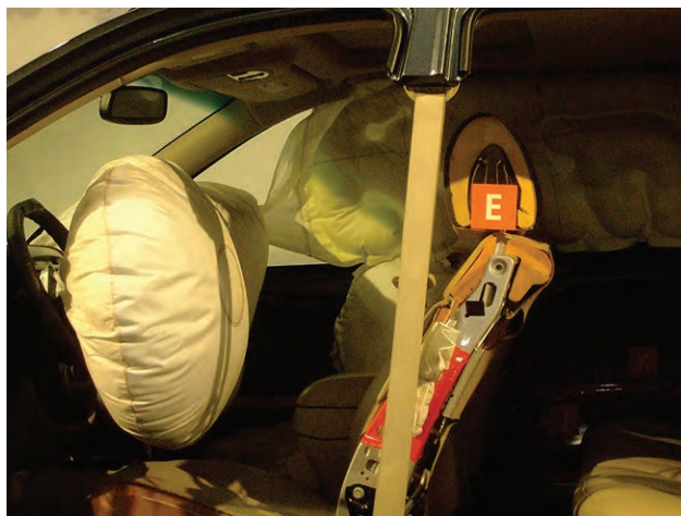
Figure 4.11 Airbags deploy upon impact to minimize serious injuries to passengers. (credit: Jon Seidman)
