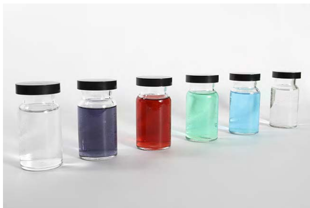
Figure 19.12 Metal ions that contain partially filled d subshell usually form colored complex ions; ions with empty d subshell ( d^0 ) or with filled d subshells ( d^{10} ) usually form colorless complexes. This figure shows, from left to right, solutions containing [M(\text{H}_2\text{O})_6]^{n+} ions with M = \text{Sc}^{3+}(d^0) , \text{Cr}^{3+}(d^3) , \text{Co}^{2+}(d^7) , \text{Ni}^{2+}(d^8) , \text{Cu}^{2+}(d^9) , and \text{Zn}^{2+}(d^{10}) . (credit: Sahar Atwa)
