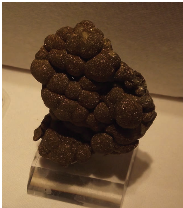
Figure 19.8 Blister copper is obtained during the conversion of copper-containing ore into pure copper. (credit: "Tortie tude"/Wikimedia Commons)
