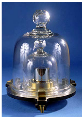
Figure 1.24 This replica prototype kilogram is housed at the National Institute of Standards and Technology (NIST) in Maryland. (credit: National Institutes of Standards and Technology)
