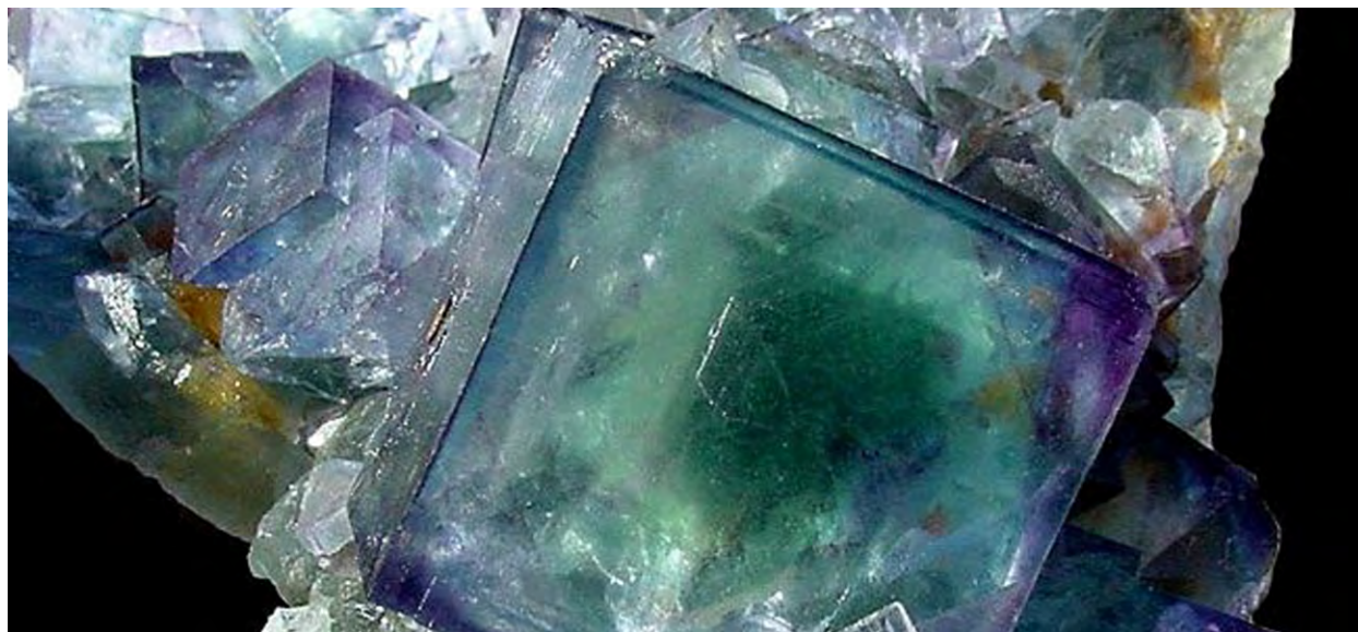
Figure 15.1 The mineral fluorite ( \text{CaF}_2 ) is deposited through a precipitation process. Note that pure fluorite is colorless, and that the color in this sample is due to the presence of other metals in the crystal.
