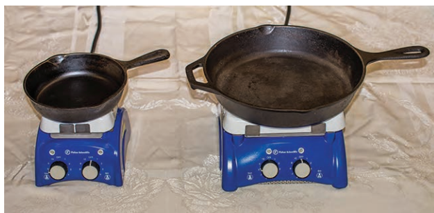
Figure 5.8 Due to its larger mass, a large frying pan has a larger heat capacity than a small frying pan. Because they are made of the same material, both frying pans have the same specific heat. (credit: Mark Blaser)
