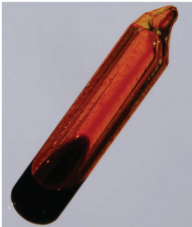
Figure 13.5 An equilibrium is pictured between liquid bromine, \text{Br}_2(l) , the dark liquid, and bromine vapor, \text{Br}_2(g) , the orange gas. Because the container is sealed, bromine vapor cannot escape and equilibrium is maintained. (credit: http://images-of-elements.com/bromine.php )
