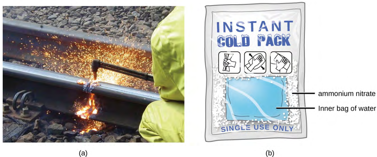
Figure 5.7 (a) An oxyacetylene torch produces heat by the combustion of acetylene in oxygen. The energy released by this exothermic reaction heats and then melts the metal being cut. The sparks are tiny bits of the molten metal flying away. (b) A cold pack uses an endothermic process to create the sensation of cold. (credit a: modification of work by “Skatebiker”/Wikimedia commons)
