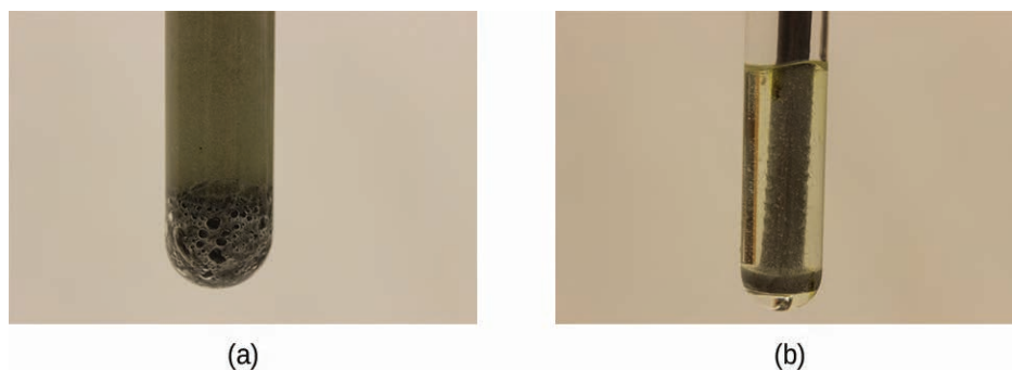
Figure 12.6 (a) Iron powder reacts rapidly with dilute hydrochloric acid and produces bubbles of hydrogen gas because the powder has a large total surface area: 2\text{Fe}(s) + 6\text{HCl}(aq) \rightarrow 2\text{FeCl}_3(aq) + 3\text{H}_2(g) . (b) An iron nail reacts more slowly.
