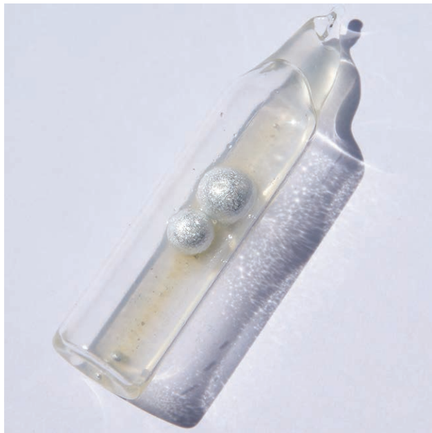
Figure 18.4 To prevent contact with air and water, potassium for laboratory use comes as sticks or beads stored under kerosene or mineral oil, or in sealed containers. (credit: http://images-of-elements.com/potassium.php )
