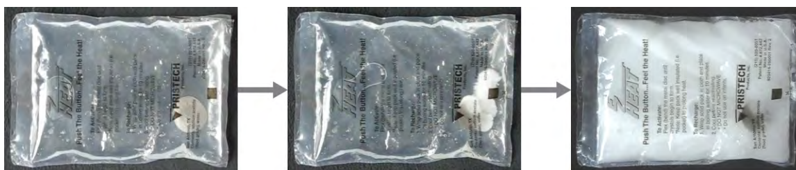
Figure 11.18 This hand warmer produces heat when the sodium acetate in a supersaturated solution precipitates. Precipitation of the solute is initiated by a mechanical shockwave generated when the flexible metal disk within the solution is “clicked.” (credit: modification of work by “Velega”/Wikimedia Commons)
