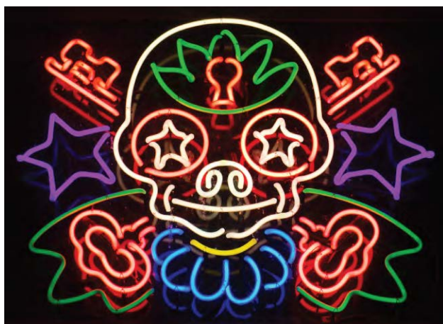
Figure 6.12 Neon signs operate by exciting a gas at low partial pressure using an electrical current. This sign shows the elaborate artistic effects that can be achieved. (credit: Dave Shaver)
