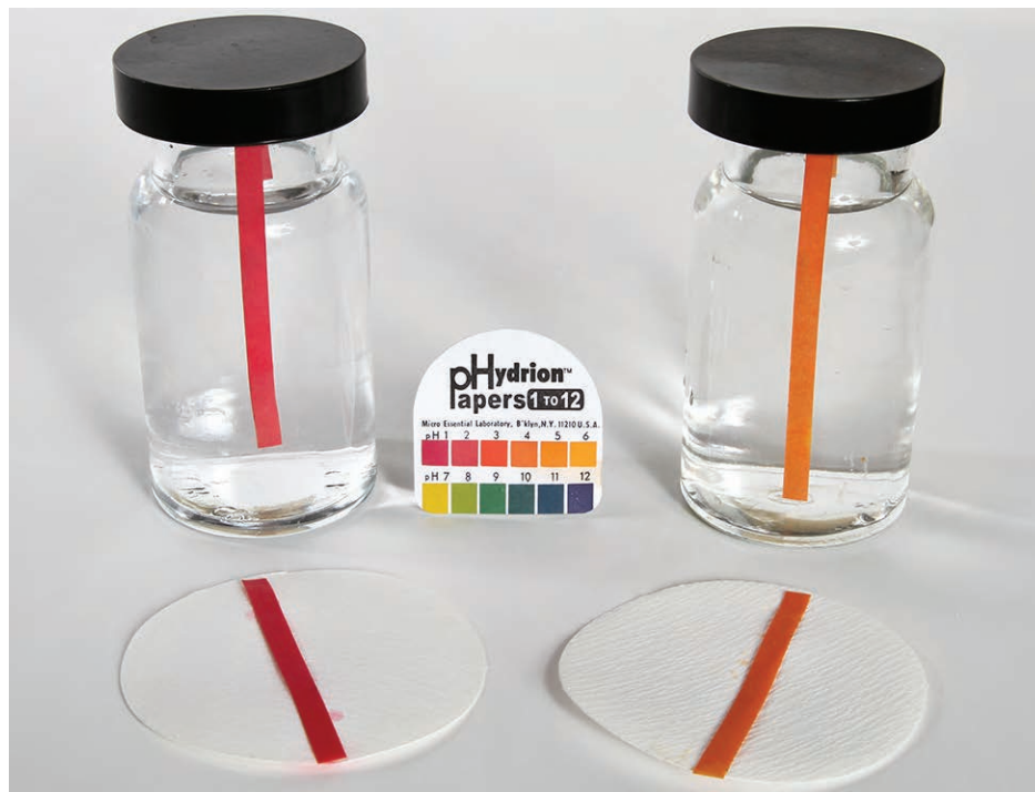
Figure 14.9 pH paper indicates that a 0.1- M solution of HCl (beaker on left) has a pH of 1. The acid is fully ionized and [\text{H}_3\text{O}^+] = 0.1\text{ M} . A 0.1- M solution of \text{CH}_3\text{CO}_2\text{H} (beaker on right) is a pH of 3 ( [\text{H}_3\text{O}^+] = 0.001\text{ M} ) because the weak acid \text{CH}_3\text{CO}_2\text{H} is only partially ionized. In this solution, [\text{H}_3\text{O}^+] < [\text{CH}_3\text{CO}_2\text{H}] . (credit: modification of work by Sahar Atwa)
