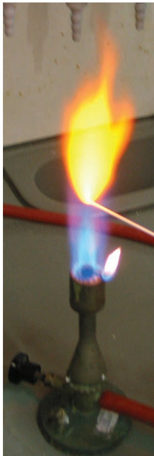
Figure 18.5 Dipping a wire into a solution of a sodium salt and then heating the wire causes emission of a bright yellow light, characteristic of sodium.
