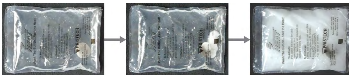
Figure 5.15 Chemical hand warmers produce heat that warms your hand on a cold day. In this one, you can see the metal disc that initiates the exothermic precipitation reaction. (credit: modification of work by Science Buddies TV/YouTube)
