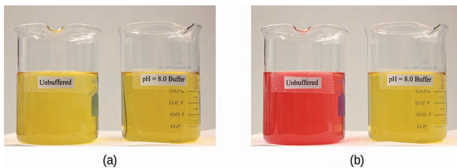
Figure 14.17 (a) The buffered solution on the left and the unbuffered solution on the right have the same pH (pH 8); they are basic, showing the yellow color of the indicator methyl orange at this pH. (b) After the addition of 1 mL of a 0.01- M HCl solution, the buffered solution has not detectably changed its pH but the unbuffered solution has become acidic, as indicated by the change in color of the methyl orange, which turns red at a pH of about 4. (credit: modification of work by Mark Ott)
