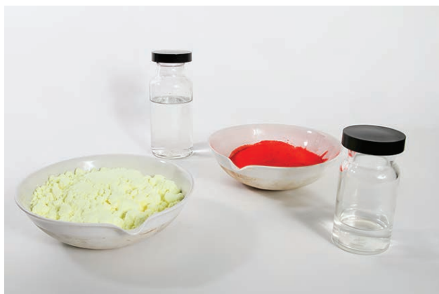
Figure 3.6 Each sample contains 6.02 \times 10^{23} molecules or formula units—1.00 mol of the compound or element. Clock-wise from the upper left: 130.2 g of \text{C}_8\text{H}_{17}\text{OH} (1-octanol, formula mass 130.2 amu), 454.4 g of \text{HgI}_2 (mercury(II) iodide, formula mass 454.4 amu), 32.0 g of \text{CH}_3\text{OH} (methanol, formula mass 32.0 amu) and 256.5 g of \text{S}_8 (sulfur, formula mass 256.5 amu). (credit: Sahar Atwa)
