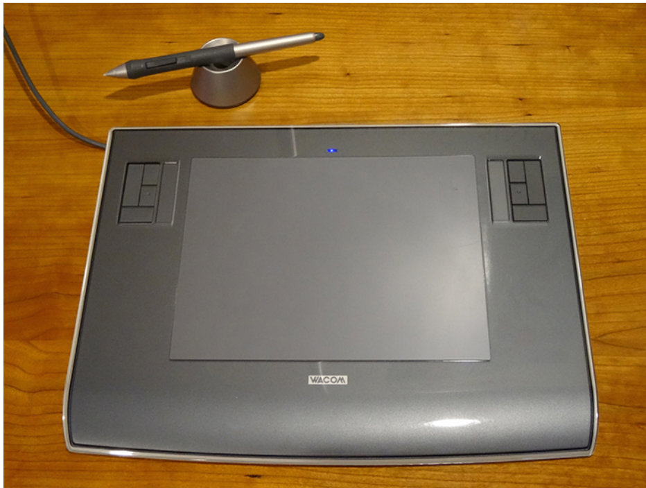
Figure 13.34 A tablet with a specially designed pen to write with is another application of magnetic induction.
