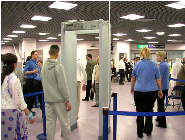
Figure 14.9 The familiar security gate at an airport not only detects metals, but can also indicate their approximate height above the floor. (credit: “Alexbuirds”/Wikimedia Commons)
