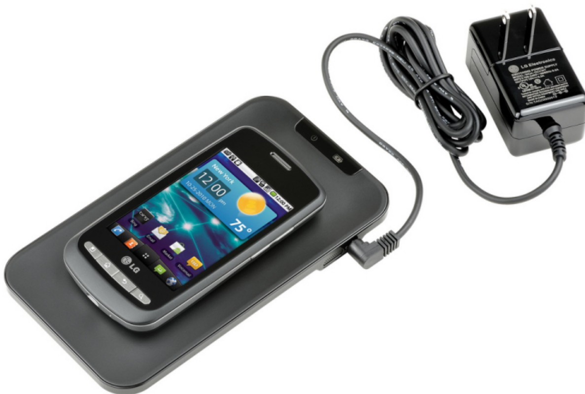
Figure 14.1 A smartphone charging mat contains a coil that receives alternating current, or current that is constantly increasing and decreasing. The varying current induces an emf in the smartphone, which charges its battery. Note that the black box containing the electrical plug also contains a transformer (discussed in Alternating-Current Circuits ) that modifies the current from the outlet to suit the needs of the smartphone. (credit: modification of work by “LG”/Flickr)
