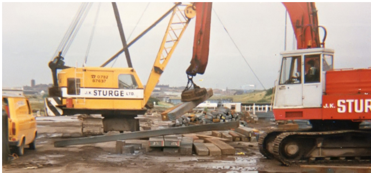
Figure 11.1 An industrial electromagnet is capable of lifting thousands of pounds of metallic waste. (credit: modification of work by “BedfordAl”/Flickr)
