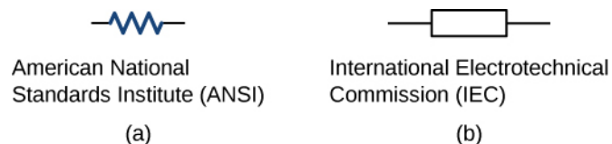
Figure 9.14 Symbols for a resistor used in circuit diagrams. (a) The ANSI symbol; (b) the IEC symbol.
