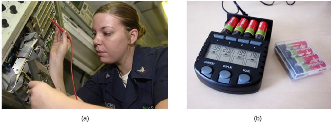
Figure 10.9 Battery testers measure terminal voltage under a load to determine the condition of a battery. (a) A US Navy electronics technician uses a battery tester to test large batteries aboard the aircraft carrier USS Nimitz . The battery tester she uses has a small resistance that can dissipate large amounts of power. (b) The small device shown is used on small batteries and has a digital display to indicate the acceptability of the terminal voltage. (credit a: modification of work by Jason A. Johnston; credit b: modification of work by Keith Williamson)
