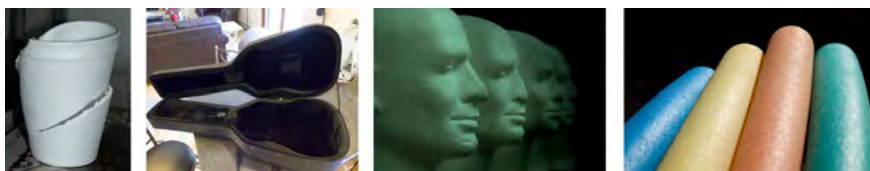
Figure 4.104: A collection of products made from polystyrene: a cup, a guitar case, polystyrene carvings, and floating pool noodles.
