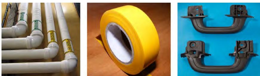
Figure 4.100: A collection of products made from polyvinyl chloride: pipes, electrical tape, and car parts.
